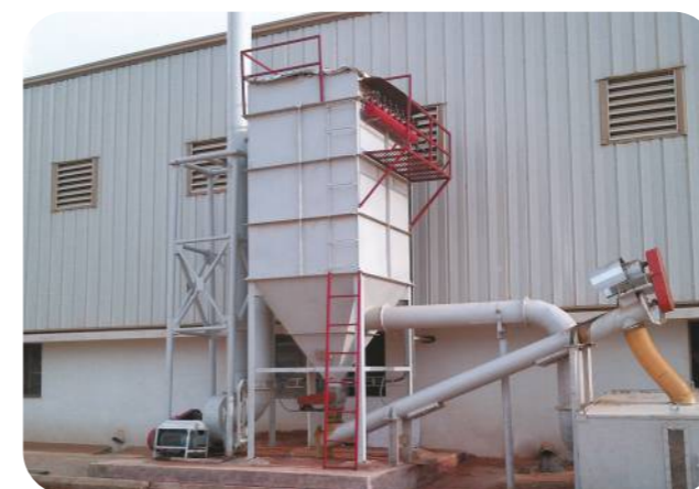
Dust Collector on Laminate Sanding
