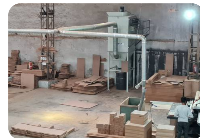
Dust Collector on Panel Saw
