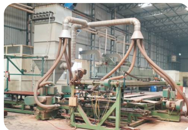
Centralized Dust Collection System for Automatic DD Saw
